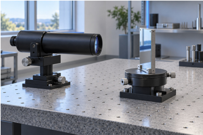
An external optical reference checks angle beyond the positioner’s internal readout.
