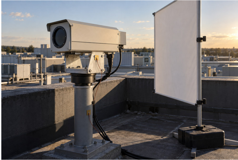
A proposed shade comparison records temperatures at the bracket and base.
