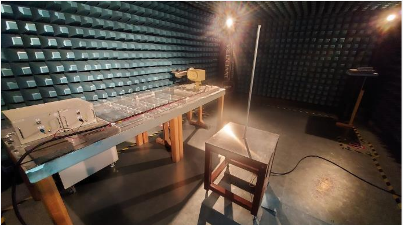
RE102 and CE102 Test Setups
