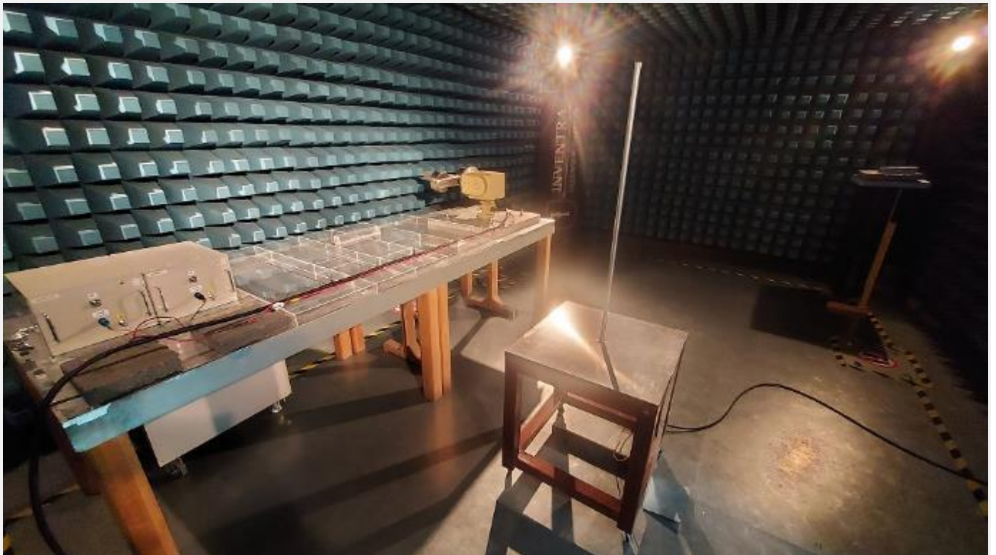
RE102 and CE102 Test Setups
